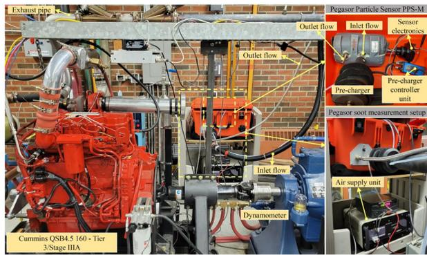
Figure 1: Diesel experimental setup
