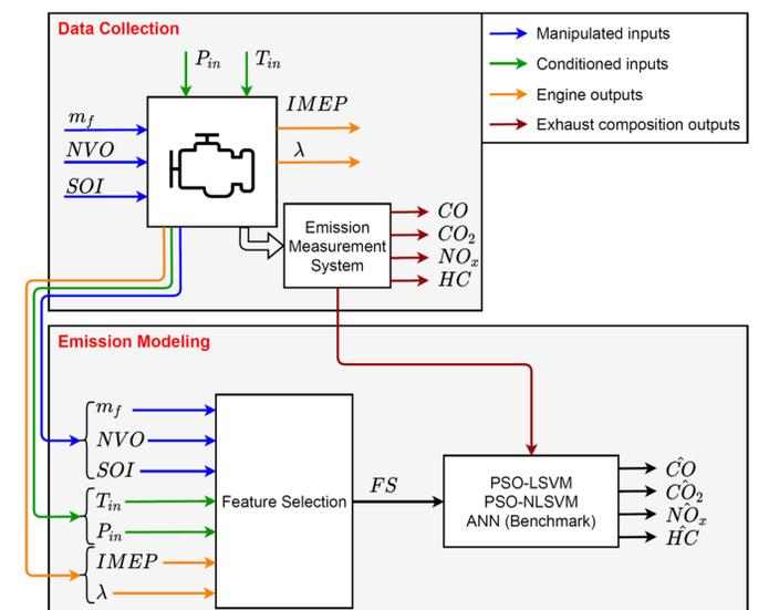
Figure 4: HCCI emission modeling process using grey-box techniques
